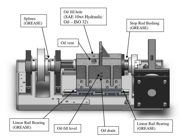
VISE CENTER – Grease monthly thru the two zerks on the front of the vise. It is recommended to use the same grease as is used on the linear bearings.
