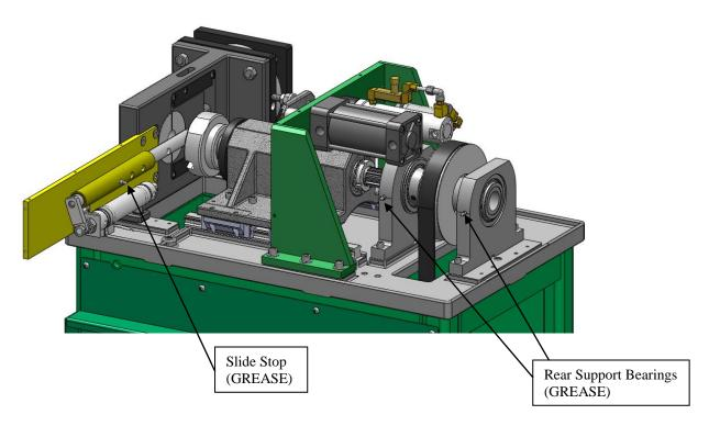
SLIDE STOP – If your machine is equipped with a slide stop it should be greased monthly thru the zerk on the slide stop. It is recommended to use the same grease as is used on the linear bearings.
