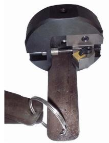
NOTE: when using the center stop rod, the same gauge is used for parts  $\frac{1}{2}$ " to  $\frac{3}{4}$ ". This is because the edge of the cutting insert is set as close to the stop rod as possible using the  $\frac{1}{2}$  -  $\frac{3}{4}$  gauge. Adjust chamfer as required by using the fine adjusting knob. Always check to see that the insert or tool holder are not rubbing the stop rod on smaller diameter settings. If required the diameter of the stop rod can be reduced on the end.
